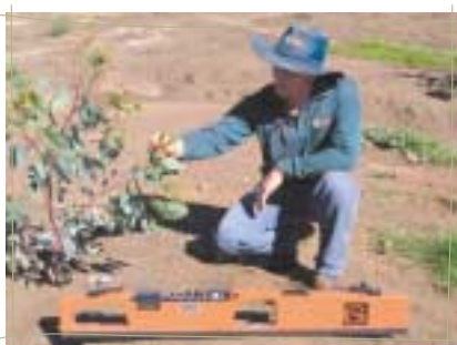
Measuring salinity with the EM38.
