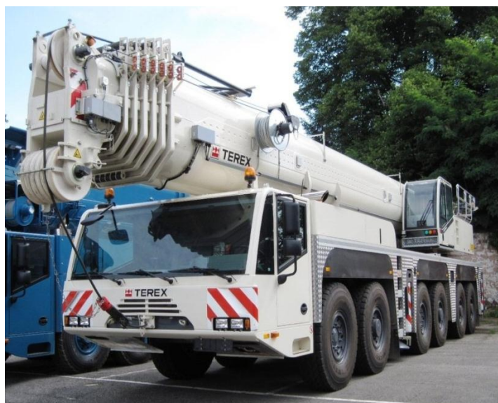
Figure 13 - New 250t crane
