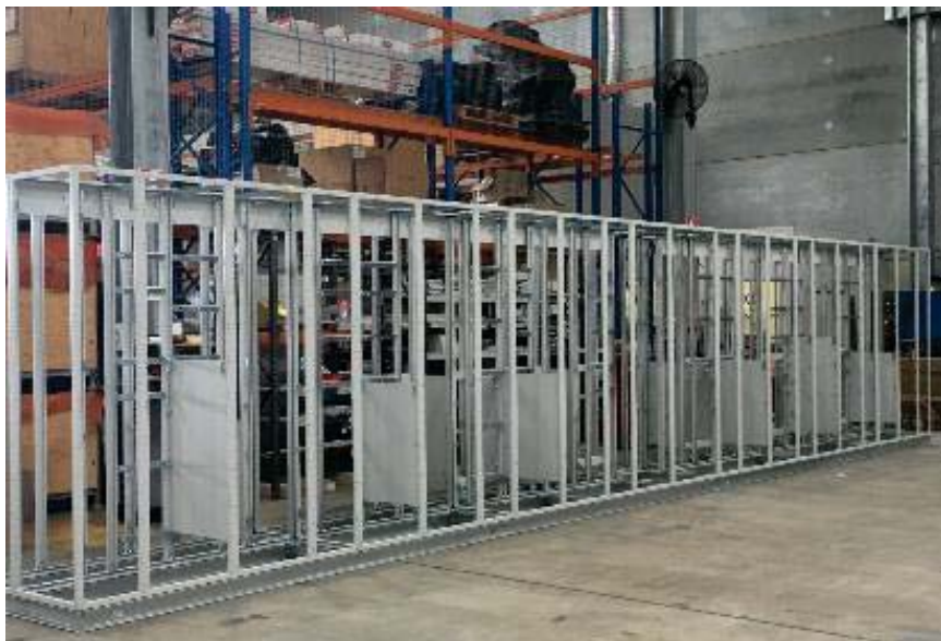
415V, 4000 Amp, 63kA, 70 starter modules, MCC frame – Pilgangoora
