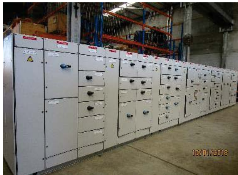
415V, 4000 Amp, 63kA, 70 starter modules, MCC frame – Pilgangoora
